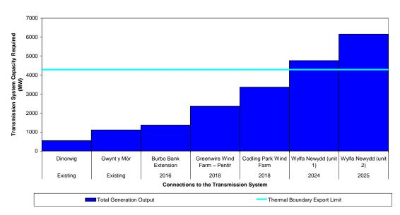
Analysis of Available Transmission Capacity [MOST ONEROUS CONDITION] Export Limits for Boundary NW3
