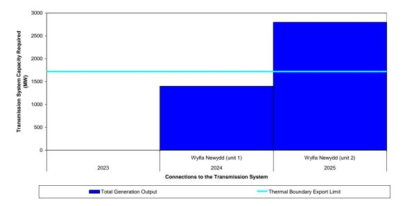
Figure 5.1: NW1 Boundary Exports. Transmission Capacity
