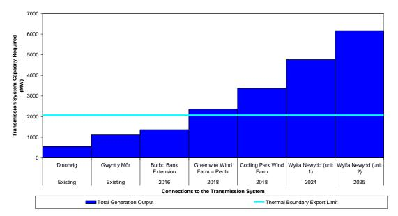
Figure 5.2: NW2 Boundary Export s. Transmission Capacity
